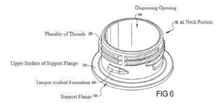
J.A. 5305. The TEF (28) in this Figure 6 embodiment is discontinuous; that is, there are multiple TEFs rather than a single, continuous formation.<sup>4</sup>
