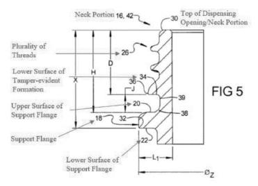
J.A. 5305. The X dimension in Figure 5 (delineated by the vertical line to the far left of the diagram) represents a measurement of the vertical distance from the top of the dispensing opening/neck portion (30) to the lower surface of the support flange (22), including the threads and a TEF. Decreasing the magnitude of the X dimension can result in lighter weight bottles and preforms, with related economic and manufacturing benefits.
