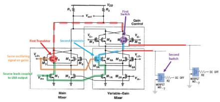
J.A. 3802. As Intel's expert explained, "one way to disable the variable-gain mixer in Der would be to turn off transistor switches M7-M10 to shut off the input signal into the gain control circuit, by setting Der's  $V_{G+}$  and  $V_{G-}$  to a low voltage (e.g. 0V)." *Id.* (capitalization normalized and emphasis omitted). This explanation for the *how* isn't remotely conclusory. J.A. 1840 ¶ 70.
