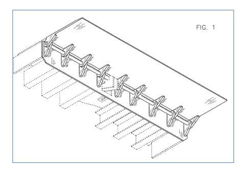
The D'754 Patent states that Figure 1 "is a perspective view showing the lip and hinge plate for a dock leveler with the lip extended, and the hinge plate secured to a deck frame shown in broken lines."
