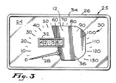
Wendt discloses a speed limit indicator which is attachable by a suction cup to the cover of a speedometer. The indicator has a pointer which is rotatable to indicate the current speed limit.
