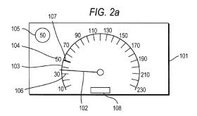
Element 105 displays a maximum speed limit, and element 107 highlights this same speed limit on the speed scale. The pointer designated by element 102 displays the vehicle's current speed.
