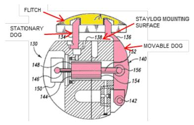
Capital's patents purport to increase the yield of veneer obtained from each log by solving problems associated with conventional methods. Most notably, the patents address problems caused by the natural taper in flitches, which occurs because trees are thicker at the base and get thinner going up the trunk. When a tapered flitch is mounted on the staylog, its outer surface is not parallel to the cutting axis of the knife. As shown below, the first
